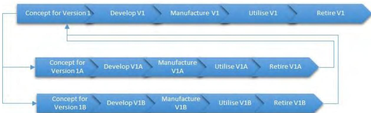
Figure 14: An example of an Experimental Approach<sup>12</sup>
